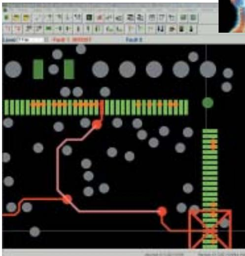
*Easy for technicians to trace a faulty net as it disappears and re emerges from inner layers*
