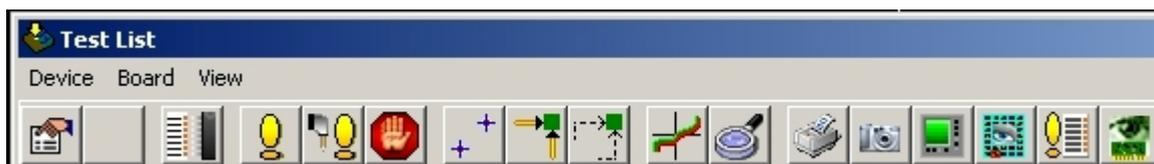
Test list mode of the GRS500 allows you to save and compare nodal impedance of a known good board against that of a board that is undergoing troubleshooting.
