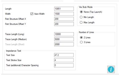
Trace Lengths for Long, Medium and Short are no longer fixed to 10 inches, 5 inches, 2 inches. They can be adjusted as follows:
