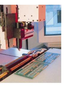
With an average test time of under 1.5 seconds, the RITS500s flying probe technology is as fast as any fixture-based impedance test system. Unlike functional bare-board test, there is no time advantage in using a fixture for RF test. What is more, a fixture-based measurement cannot be verified at the probe tip.
