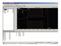
a simple display of impedance versus distance, and reports a PASS or FAIL for each test.
