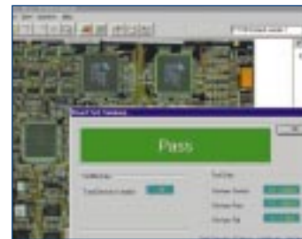
The FT100 uses impedance comparison techniques to help you faultfind complex pcbs.
